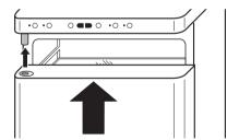
Slide the centre door bearing into the bottom left of the fridge compartment door and fasten to the housing.
